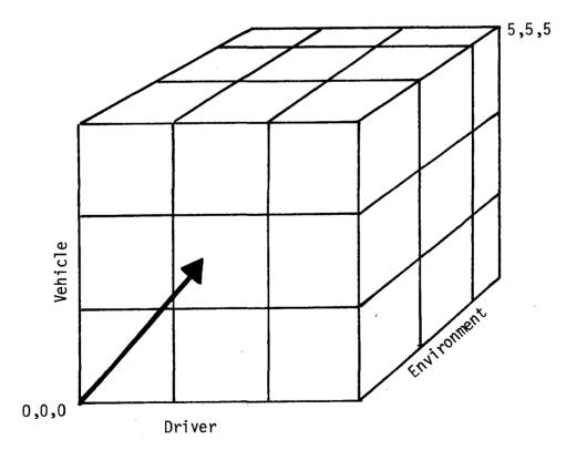
Accidents receiving an 0,0,0 rating were, of course, the most benign accidents, while accidents considered to have a 5,5,5 rating would indicate total system failure. The vast majority of the cases fell somewhere in the interior of the three-dimensional cube. The distance of the ray measured from the 0,0,0 origin is defined as the amount of estimated system failure in each individual accident is calculated by the following formula:
