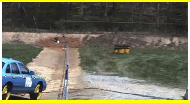
CABLE SHOULD NOT BE PLACED BETWEEN 1' AND 8' BEYOND THE BOTTOM OF A DITCH
