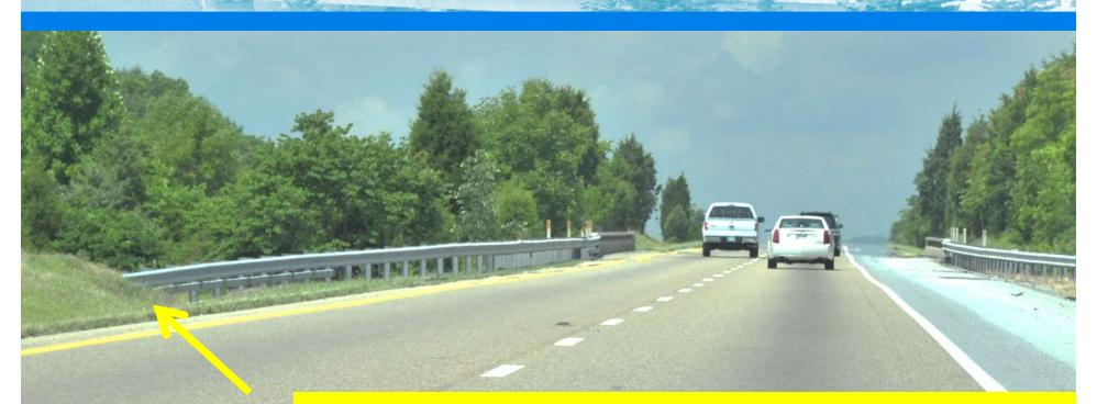
The point where the BIC crosses the toe of the backslope must be far enough upstream of the hazard. Top rail must capture vehicle
